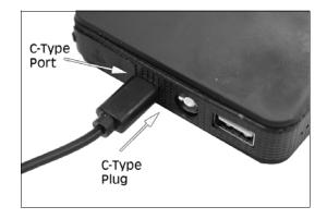
The BLUE charging/indicator lights on the jump starter will come on and start flashing to indicate charging is in progress.
